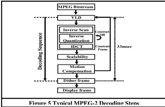
Figure 5 Typical MPEG-2 Decoding Steps
