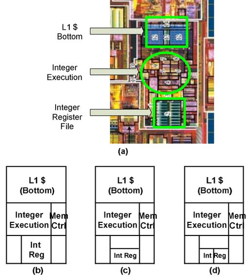
**Figure 4 Detailed Floor-plan for the Register File**
